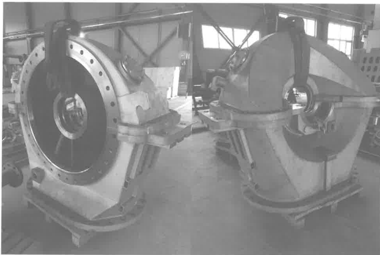
Fig. 14: Exhaust of the modernized 101JT steam turbine (1950 of t/day)
