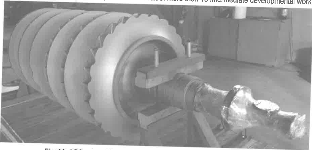
Fig. 11: LPC rotor of the modernized 101J air compressor (1950 of t/day)
